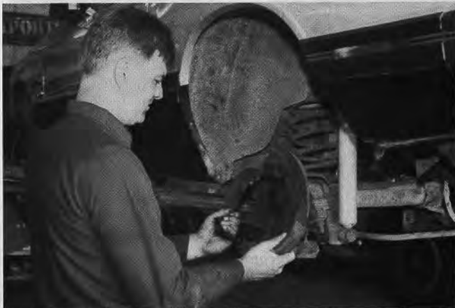
Removal of the shoes and hardware from the old drum rear brake system is the first step. SSBC's conversion kit uses the original brake lines and offers a connection for the parking brake as well.
