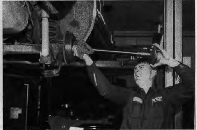
With the C-clips removed, sliding the axle shafts out is a pretty easy job. This is a great time to inspect the axles for signs of wear and replace the axle bearings and seals, too.
