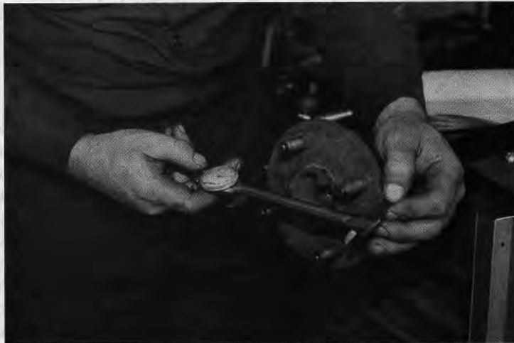
SSBC uses a special one-piece casting of their own design to mount the calipers which makes this conversion possible. Brackets are different on each side of the car and are marked accordingly.
