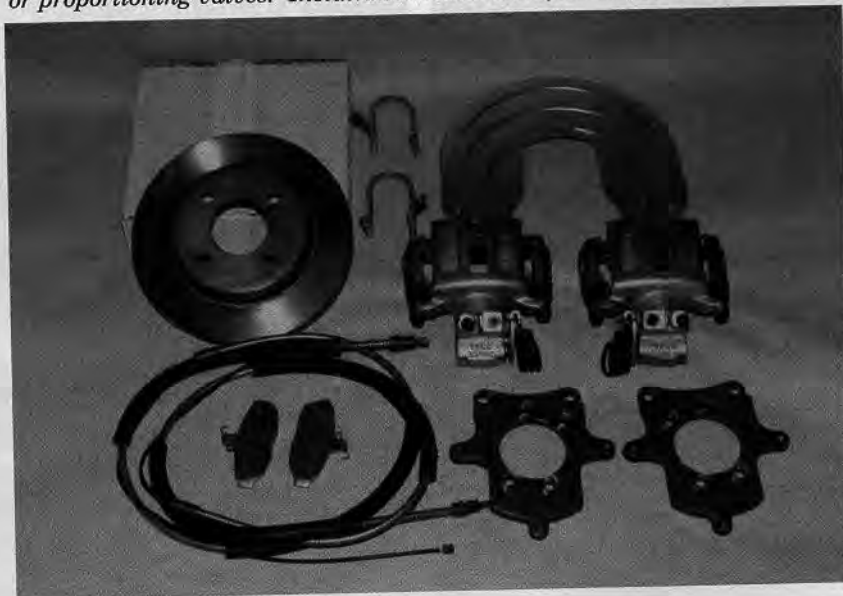
Rear disc brake conversion kits can be very simple. This kit for 1979-86 Mustangs doesn't need a replacement master cylinder, distribution blocks, or proportioning valves. Installation time takes four to five hours.
