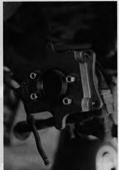
SSBC uses a special one-piece casting of their own design to mount the calipers which makes this conversion possible. Brackets are different on each side of the car and are marked accordingly.
