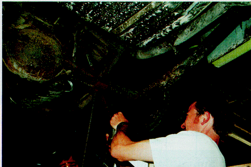
4) When removing rear leaf springs, always be sure to support the rear axle as the rear springs supports the rear axle housing. Failure to do so can result in significant injury.
