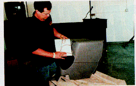
Classic Design Concepts is well known for their light bars. A template is used to mark the exact location for cutting of the interior quarter panel. Professionals make installation appear very easy.
