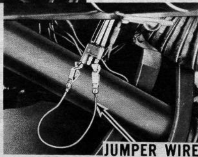
Figure 4—Jumper Wire For Switch Wiring
