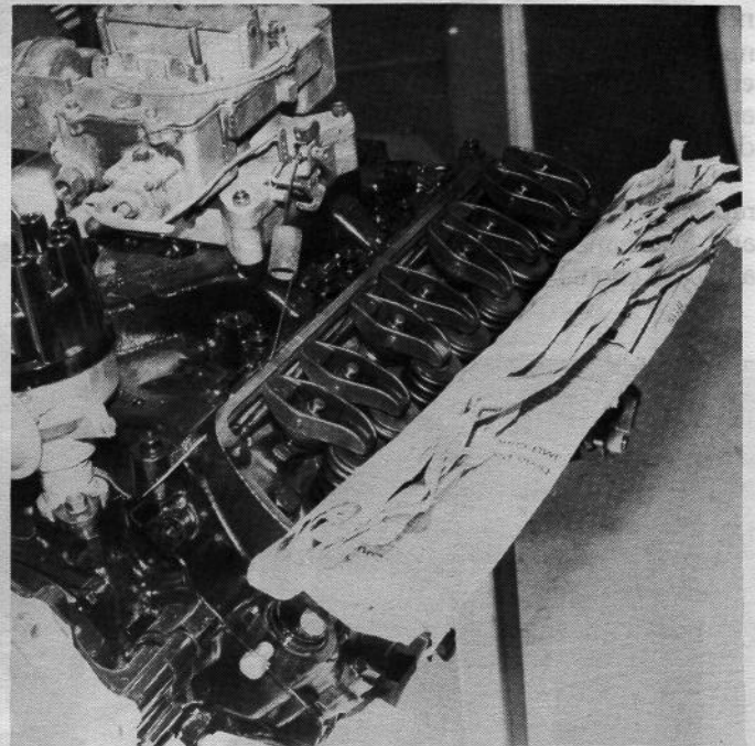
4. Folded newspaper prevents oil from splashing on fender wells.
