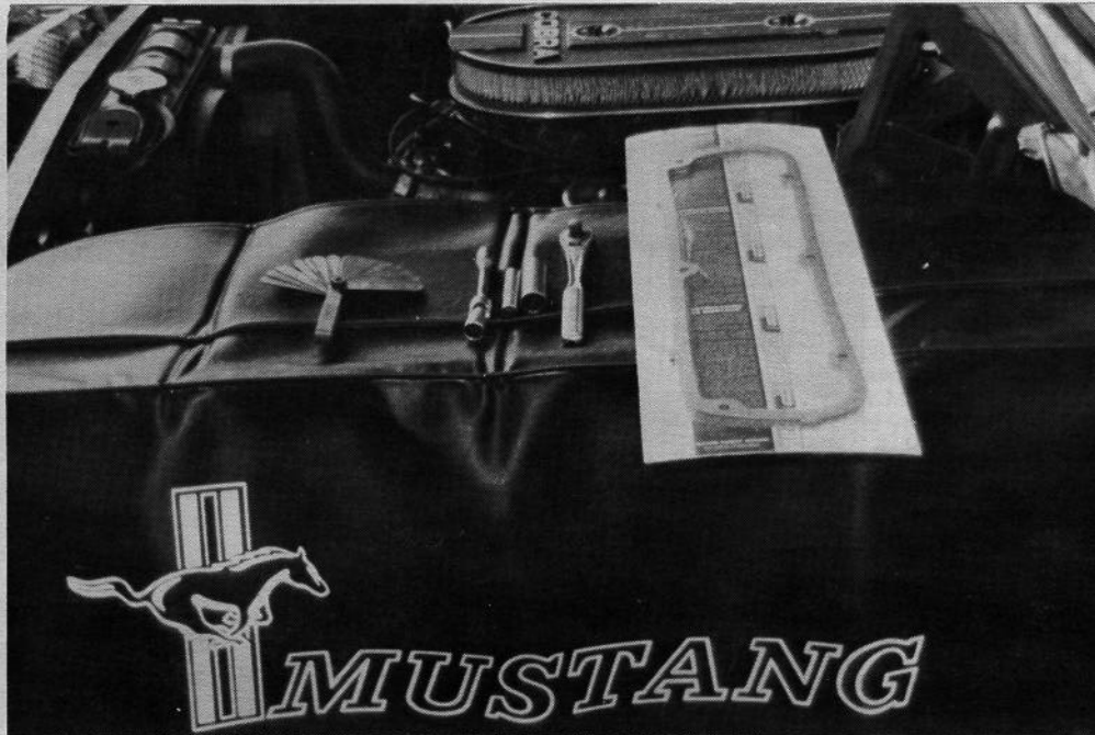
2. Tools necessary for the job: from left — feeler gauges to measure clearance, sockets and ratchet, new valve cover gaskets, and a fender cover (Mustang type of course) to protect the finish.
