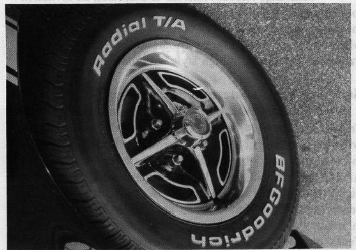
Styled steel wheels and Radial T/As greatly enhance handling. Original equipment was the Firestone Steel Radial 500 tire.
