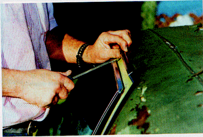
Removing the exterior trim is the first step in removing a vinyl top. Use a flat blade screwdriver to carefully lift metal and explore to locate the clips as shown here. This Mustang also had bolts at various places that could only be accessed by removing the headliner.
