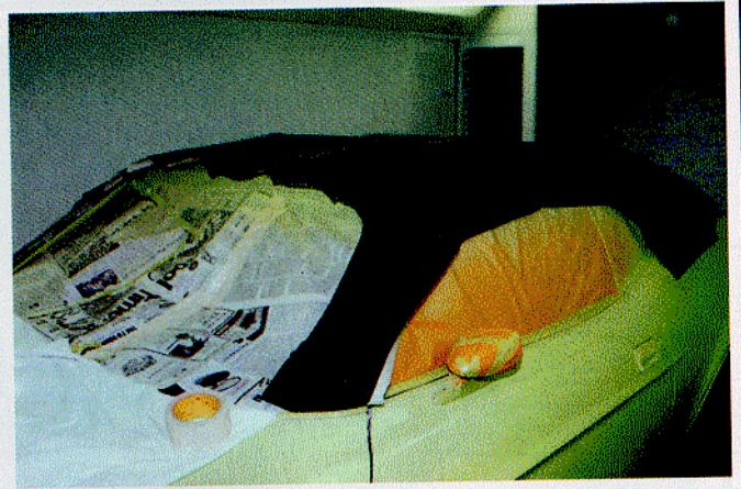
Prior to installation, the new vinyl roof was laid out over the car's top and carefully marked so it could be properly positioned once the cement was applied. Note that the windshield was removed and all glass was covered as protection from overspray when the roof was painted.
