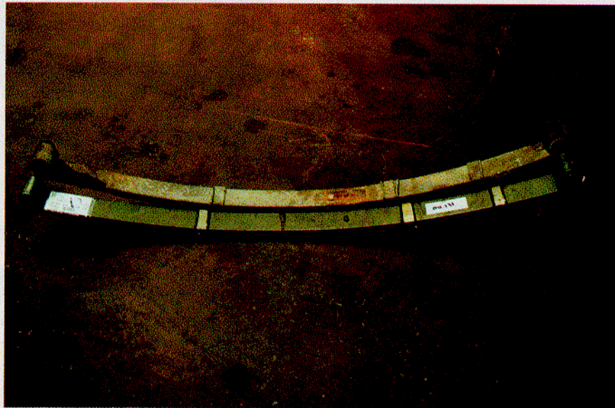
1) An on-the-floor comparison of the old (top) and new springs (bottom) showed that the replacements had substantially more arch than what came off the car.
