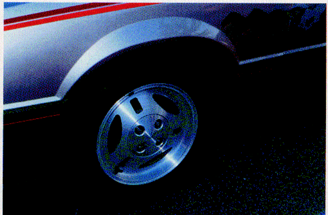
5) Although they looked good, TRX forged aluminum wheels (made between 1979-84) aren't seen much anymore probably due to their metric size which require Michelin tires that usually need to be special ordered.
