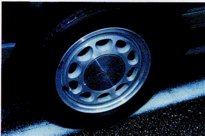
4) Beginning in 1985, these cast aluminum wheels came standard on Mustang GTs and some late production LX cars as well. Known as "ten-holes", these 15 x 7-inch wheels have an offset of 4.875 inches.
