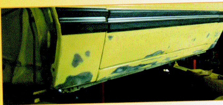
Of greater concern initially were the bubbled areas around the rocker panels, rear wheel openings and quarter panel. Removing the paint, revealed little more than surface rust, but the area was treated and then repainted to keep this problem from spreading.
